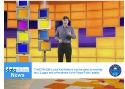
Luma Keyed Image with Background Video showing through the Black Matte Area
